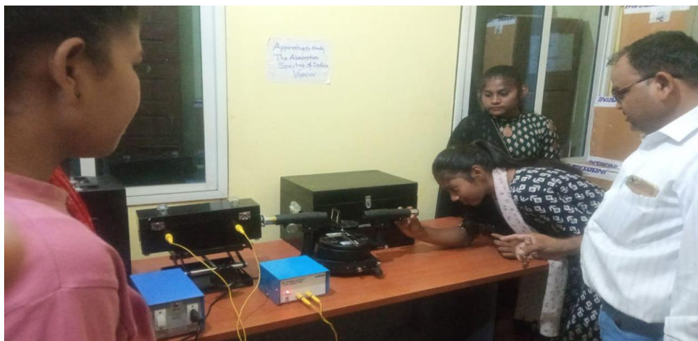
Fig : Laboratory work of Physics Students using Absorption Spectrum Of Iodine Vapour Using Spectrometer
